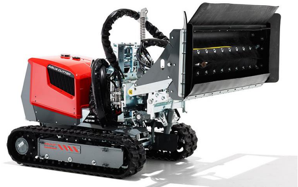
Figure 2 - AquaJet Aqua Cutter is a remote controlled and telescoping hydro demolition equipment to be utilized for cover concrete removal
